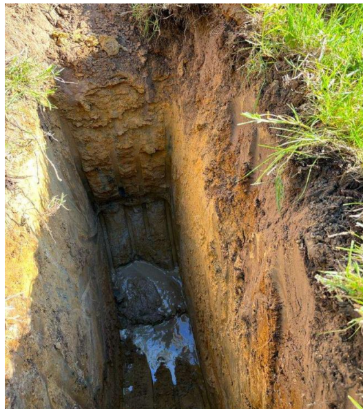
Figure 2: Photo of geotechnical test pit on site showing orange clayey sand at depth.
